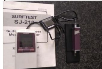
Gambar 5. Surface Roughness Tester
