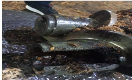
Gambar 2. Worm screw pecah
