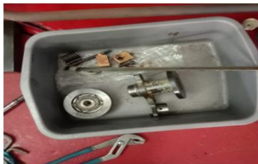
Gambar 4.5 Proses pembongkaran Cross screw
