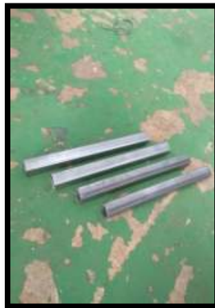
Gambar 2. Material Baja St37 Hollow
